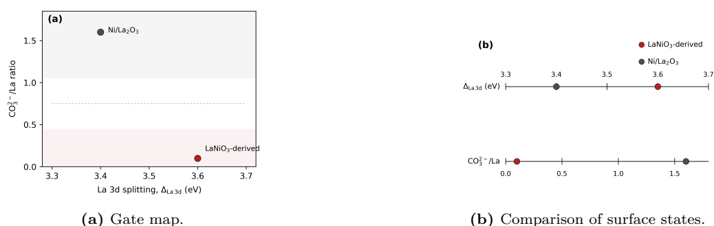
Figure 4. Surface-characterisation parameters used for distinguishing between open hydroxide/oxycarbonate-compatible and blocked carbonate-containing interfaces. Perovskite-derived reaction surface is characterized by a 3.6 eV La 3d splitting and low carbonate abundance, while impregnated Ni/La 2 O 3 surface is characterized by a 3.4 eV splitting and high carbonate abundance.
