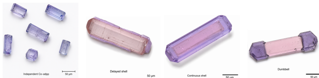
(a) Rejected Co–adpp growth. (b) Delayed shell condition. (c) Conformal shell condition. (d) Terminal dumbbell condition.
